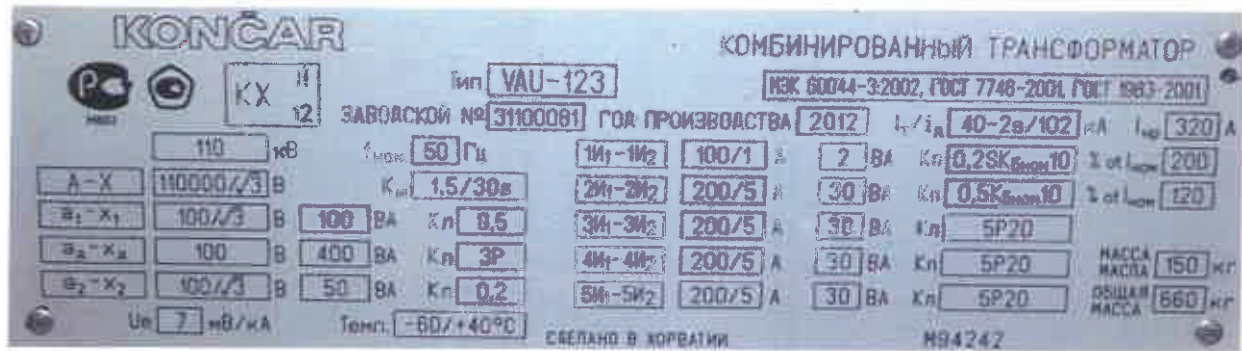
Figure 1. Photo of The AGU-123 identification plate
