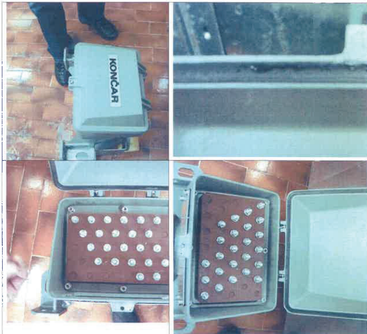
Picture 8: Results of water resistance test on the EUT
