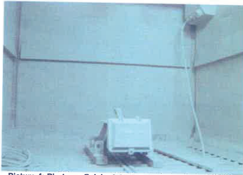
Picture 4: Photo on finish of dust resistance test on the EUT
