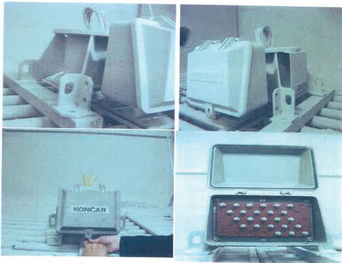
Picture 4: Photo on finish of dust resistance test on the EUT
