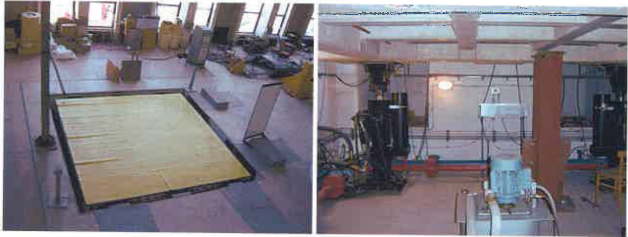
Figure 12: IZIS' seismic shaking table – top view on the left, below the table on the right
